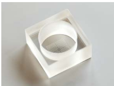
The Embryo Immobilisation Chip enables high resolution imaging of embryos.
